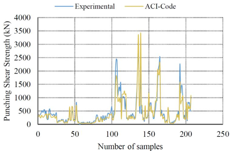
Figure 9. Experimental and predicted punching shear strength for all samples.
