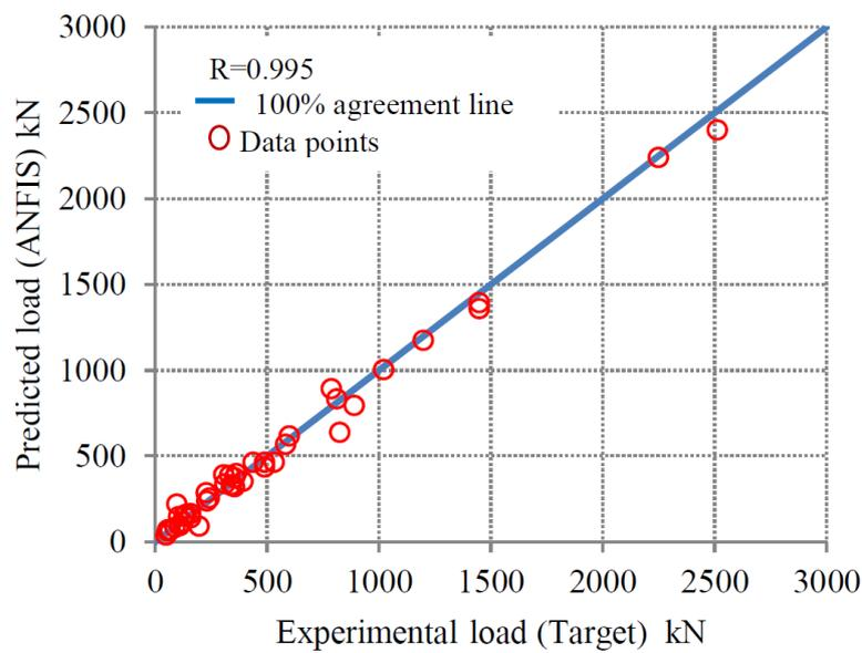
Figure 5. Experimental and predicted punching shear strength (testing dataset).
