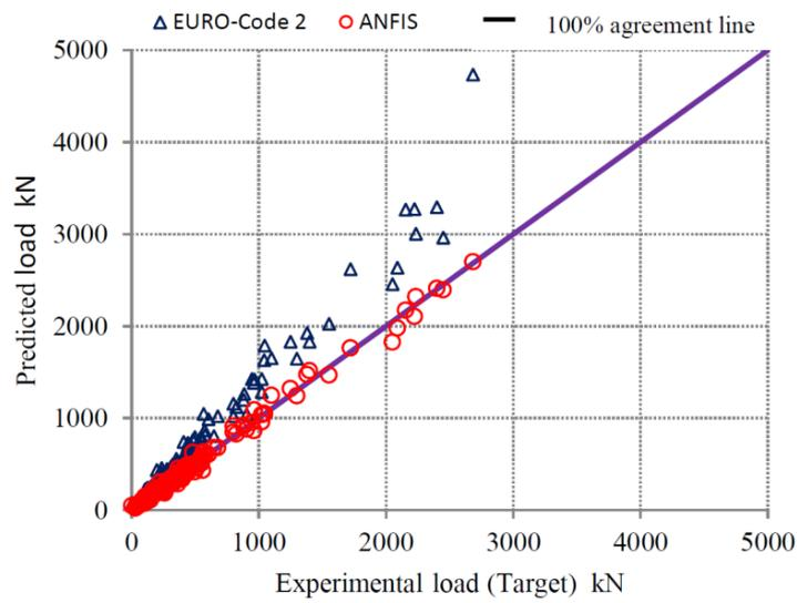
Figure 16. Experimental and predicted punching shear strength (training dataset).
