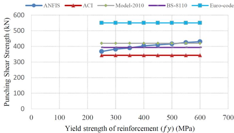
**Figure 23.** Effect of yield strength of reinforcement on the punching shear strength.
