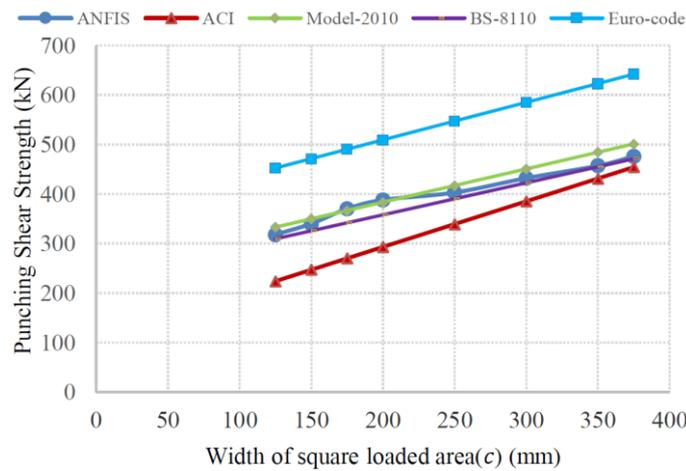
Figure 21. Effect of width of square loaded area on the punching shear strength.
