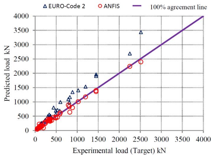
Figure 17. Experimental and predicted punching shear strength (testing dataset).
