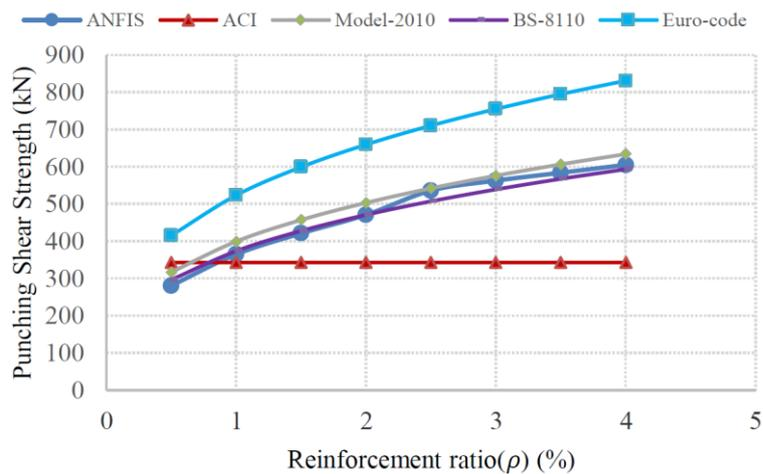
Figure 22. Effect of the reinforcement ratio on the punching shear strength.
