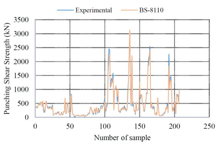
Figure 15. Experimental and predicted punching shear strength for all samples.
