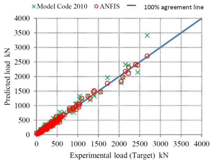
Figure 10. Experimental and predicted punching shear strength (training dataset).
