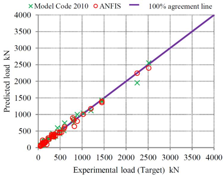
Figure 11. Experimental and predicted punching shear strength (testing dataset).
