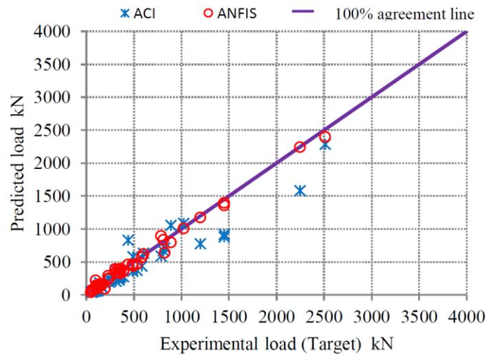
Figure 8. Experimental and predicted punching shear strength (testing dataset).
