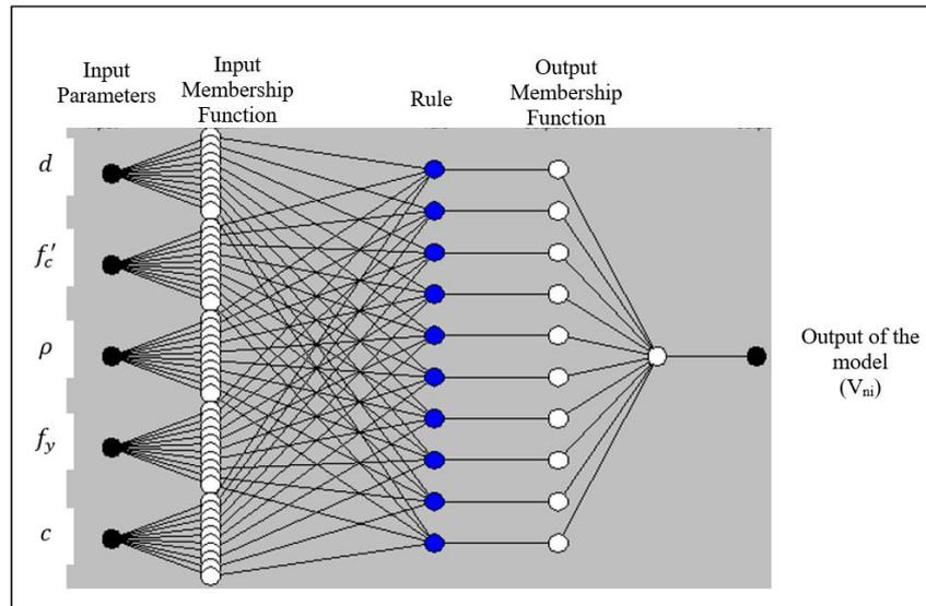
Figure 2. Network Structure of the ANFIS model.
