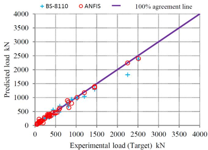
Figure 14. Experimental and predicted punching shear strength (testing dataset).
