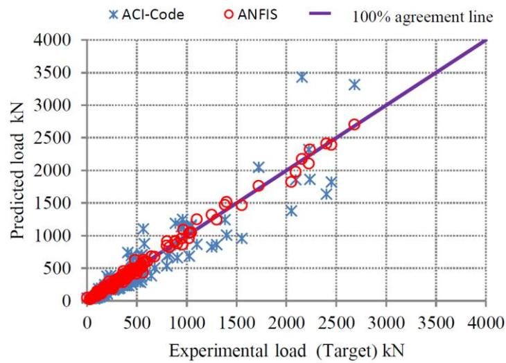
Figure 7. Experimental and predicted punching shear strength (training dataset).
