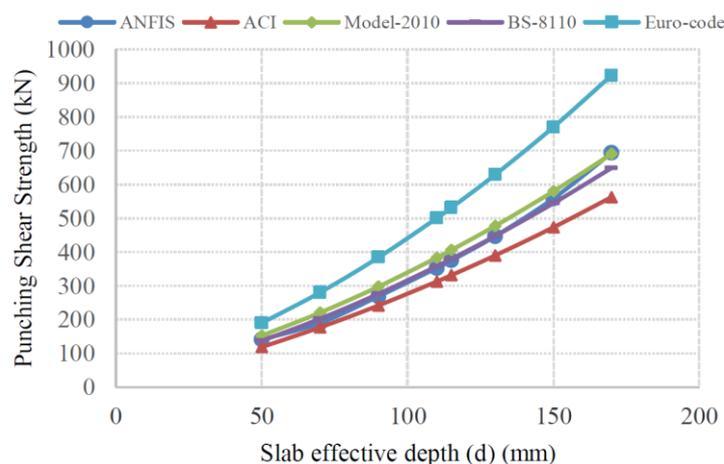
**Figure 19.** Effect of slab effective depth on the punching shear strength.
