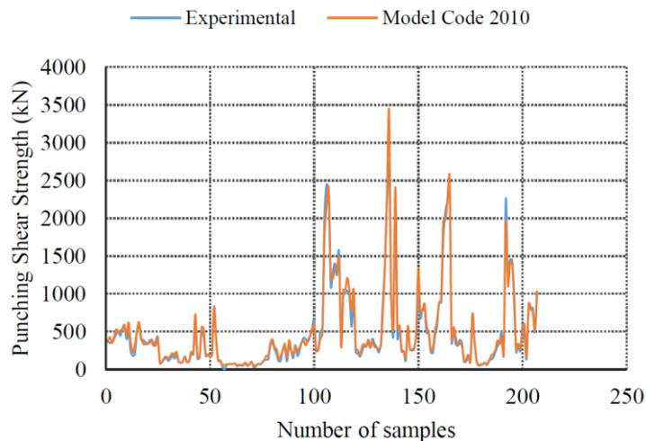
Figure 12. Experimental and predicted punching shear strength for all samples.
