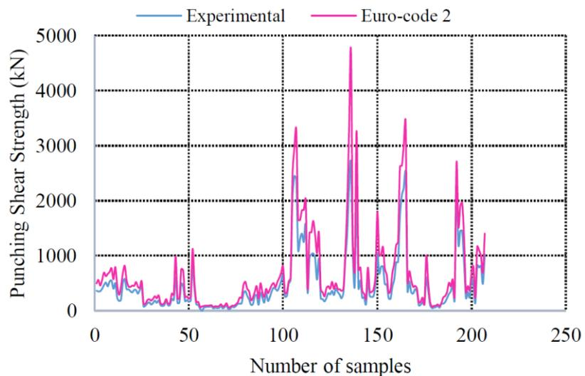
Figure 18. Experimental and predicted punching shear strength for all samples.
