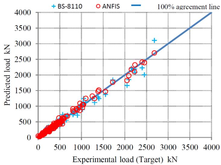
Figure 13. Experimental and predicted punching shear strength (training dataset).
