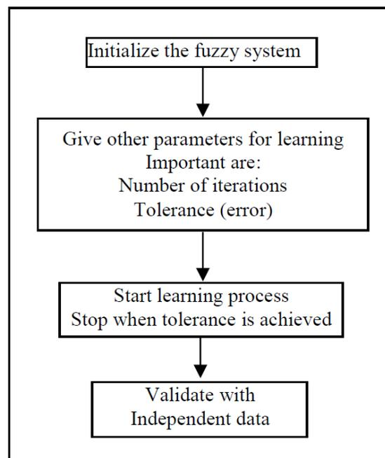
**Figure 1.** The basic flow diagram for computations in an adaptive neuro-fuzzy interface system (ANFIS).
