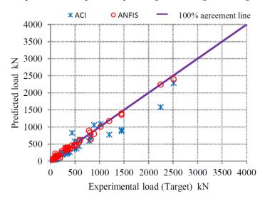
Figure 8. Experimental and predicted punching shear strength (testing dataset).
