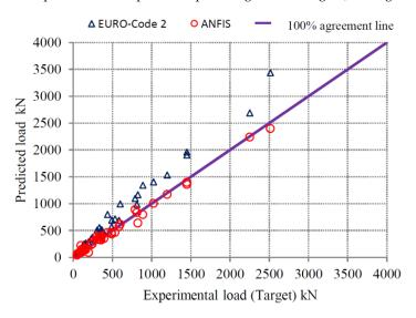
Figure 17. Experimental and predicted punching shear strength (testing dataset).
