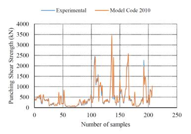
Figure 12. Experimental and predicted punching shear strength for all samples.
