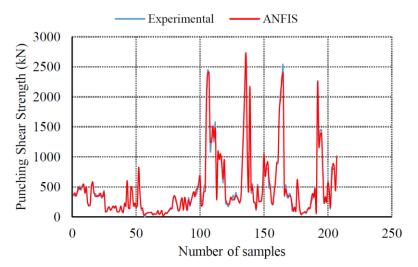
Figure 6. Experimental and predicted punching shear strength for all samples.
