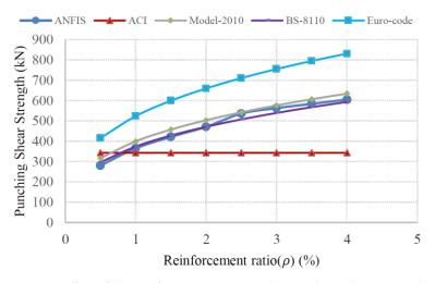
Figure 22. Effect of the reinforcement ratio on the punching shear strength.
