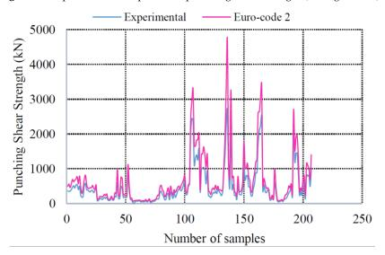
Figure 18. Experimental and predicted punching shear strength for all samples.
