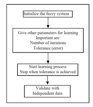
**Figure 1.** The basic flow diagram for computations in an adaptive neuro-fuzzy interface system (ANFIS).
