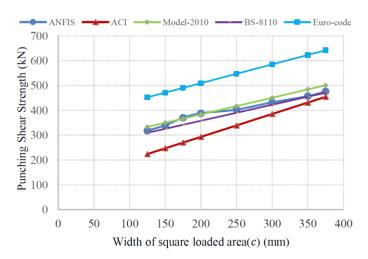
Figure 21. Effect of width of square loaded area on the punching shear strength.
