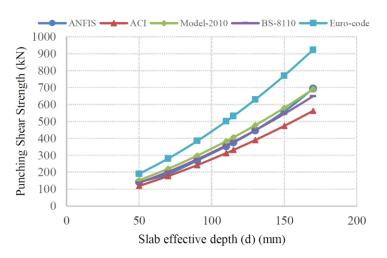
Figure 19. Effect of slab effective depth on the punching shear strength.
