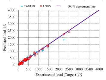
Figure 14. Experimental and predicted punching shear strength (testing dataset).
