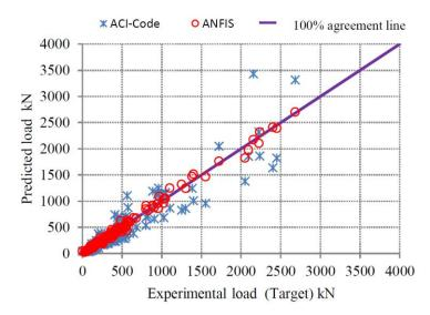
Figure 7. Experimental and predicted punching shear strength (training dataset).
