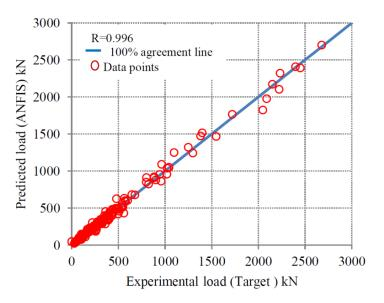
Figure 4. Experimental and predicted punching shear strength (training dataset).
