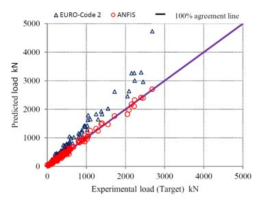
Figure 16. Experimental and predicted punching shear strength (training dataset).
