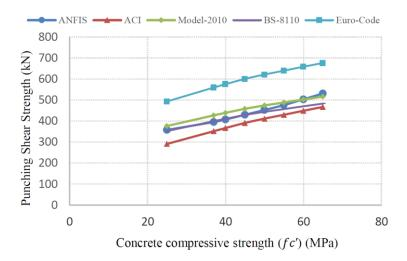
Figure 20. Effect of concrete compressive strength on the punching shear strength.
