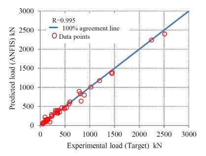
Figure 5. Experimental and predicted punching shear strength (testing dataset).
