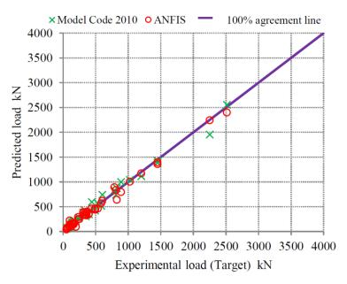
Figure 11. Experimental and predicted punching shear strength (testing dataset).
