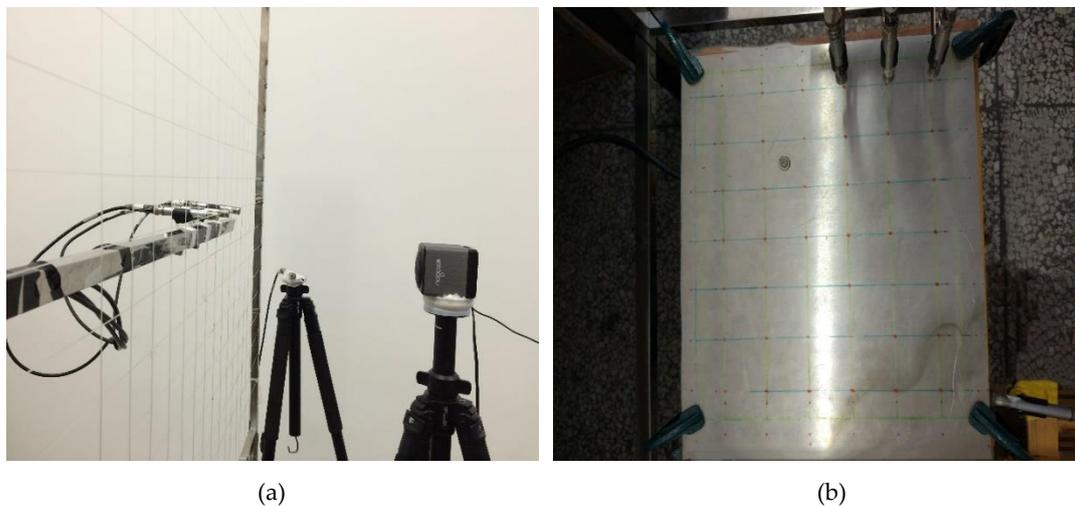
**Figure 9.** Experimental setup: (a) Single source; (b) Plate sound source.
