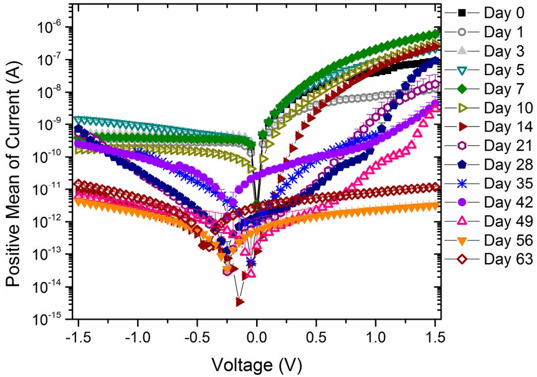
**Figure S2.** Complete set of *I-V* curves of a single SiNW measured before and after immersion in PBS at 37 °C for the given time period. Data points represent the mean and standard deviation of three measurements.
