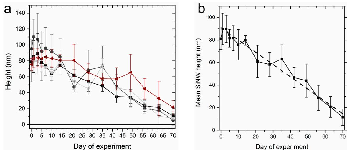
**Figure S1.** The height of four SiNWs over immersion time in PBS at 37 °C (a), each curve corresponding a single SiNW. Each data point corresponds to the mean of at least 2, usually 4–6, height measurements at different locations along the wire. In (b) the mean over all measured height profiles of all SiNW was fitted linearly. The slope yields an estimate for the SiNW etching rate under said conditions of  $(1 \pm 0.1)$  nm/day.
