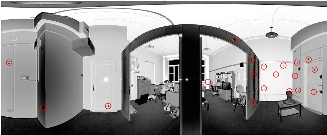
**Figure 7.** The example of the point cloud in the spherical projection of test site III: “The office room” with marked check points (red circles).
