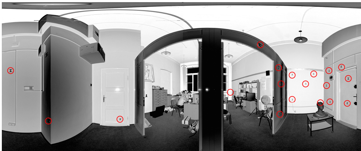
Figure 7. The example of the point cloud in the spherical projection of test site III: “The office room” with marked check points (red circles).
