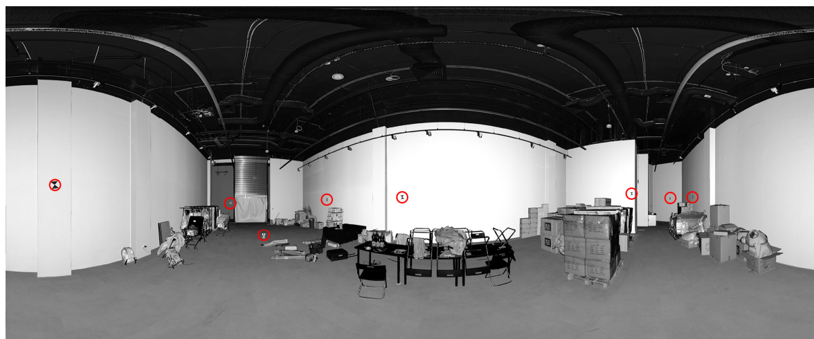
Figure 9. The example of the point cloud in the spherical projection of test site IV: “Empty shop (shopping mall)” with marked check points (red circles).
