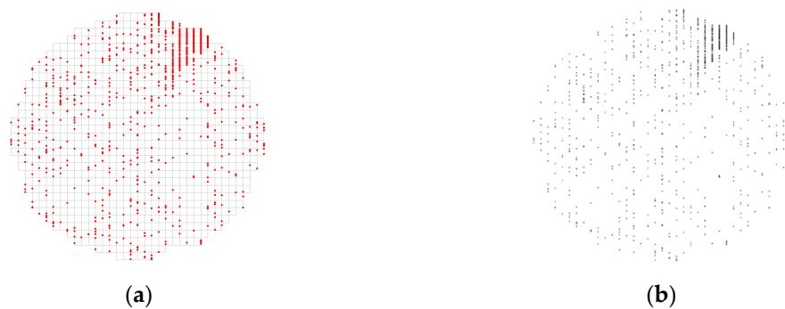
Figure 3. (a) Construction of wafer bin map image; (b) preprocessed image from (a).
