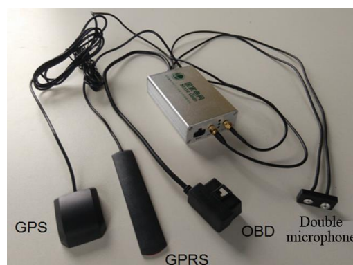
Figure 2. Object of time-sharing rental vehicle terminal for electric vehicle based on acoustic communication technology.
