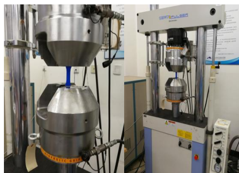
Figure 3. Tensile test machine (servo-hydraulic) and the sample.
