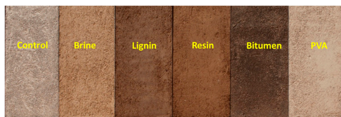
Figure 2. The soil samples in trays after the application of the dust control product used for the laboratory wind tunnel experiment. The size of each tray is 0.5 \times 1.0 m with height of 0.02 m. each soil sample was prepared in three replicates.
