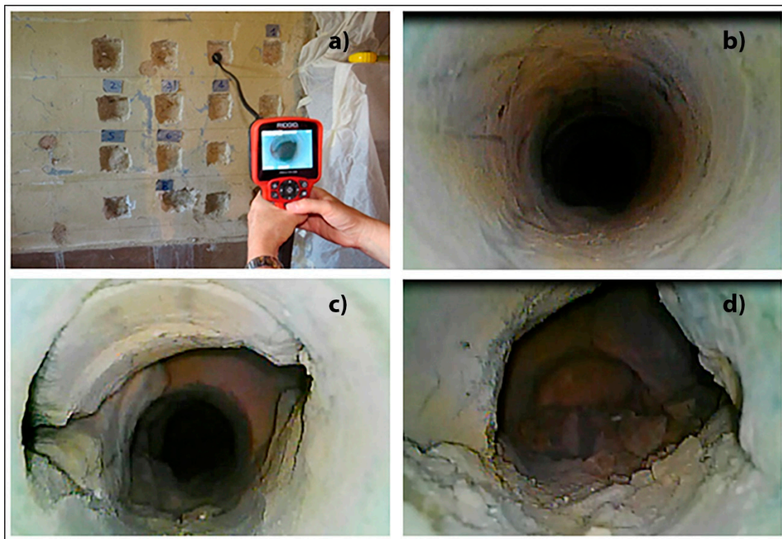
Figure 5. (a) Endoscopy surveys; (b) Initial section of compact masonry; (c) First discontinuity; (d) Central discontinuity between two walls.
