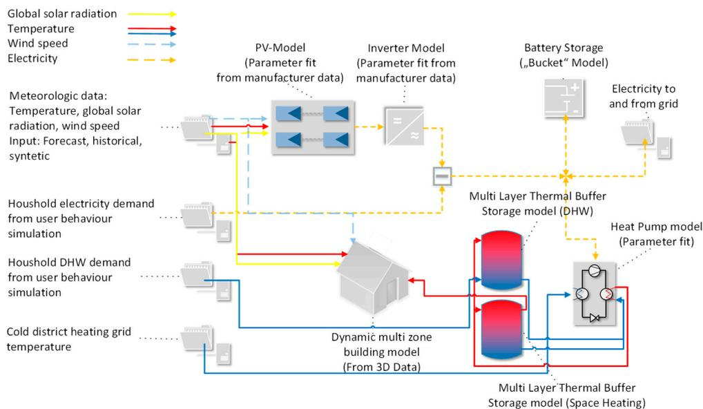
**Figure 12.** Integrated white box INSEL model combining a dynamic building model and energy conversion systems.
