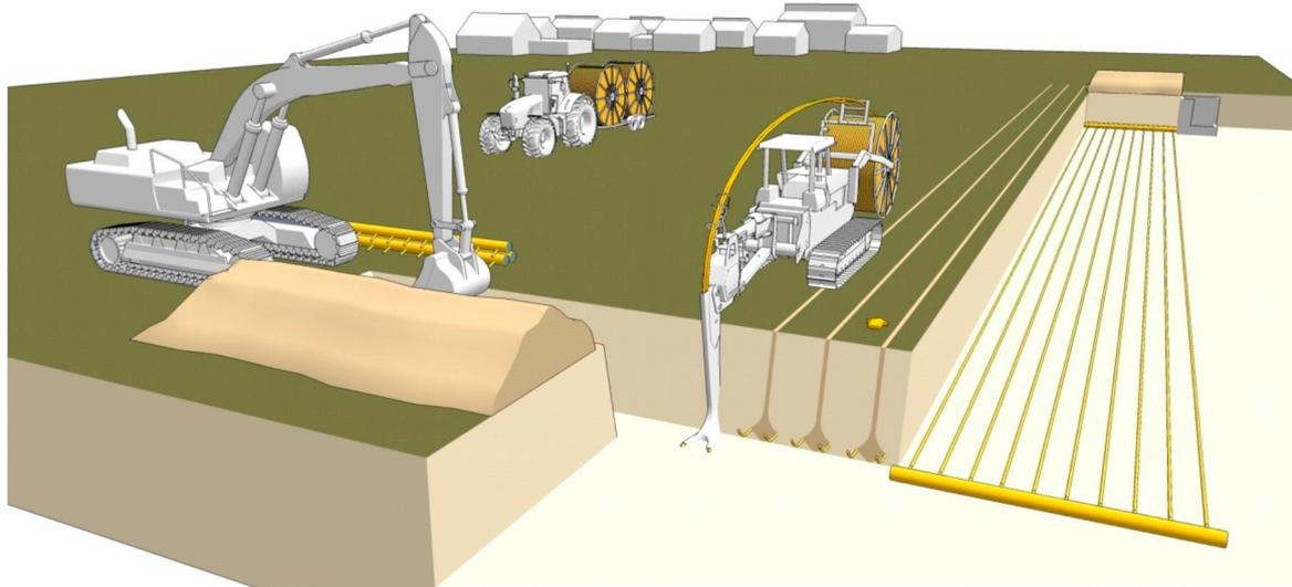
Figure 3. Installation of the agrothermal collector field (under approval of Doppelacker GmbH).
