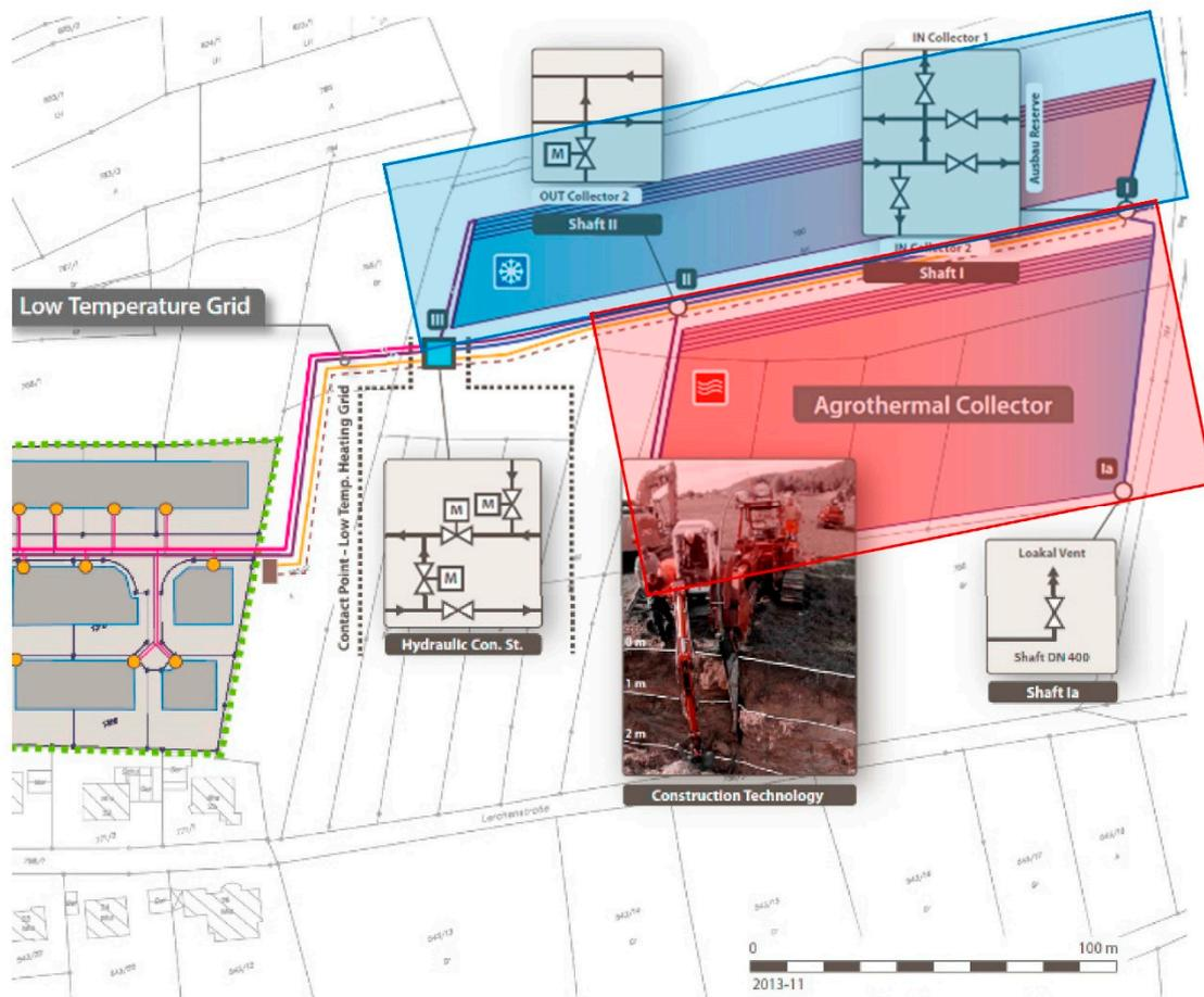
**Figure 2.** Low-temperature DHC network with realized (blue) and planned (red) collector construction phases.
