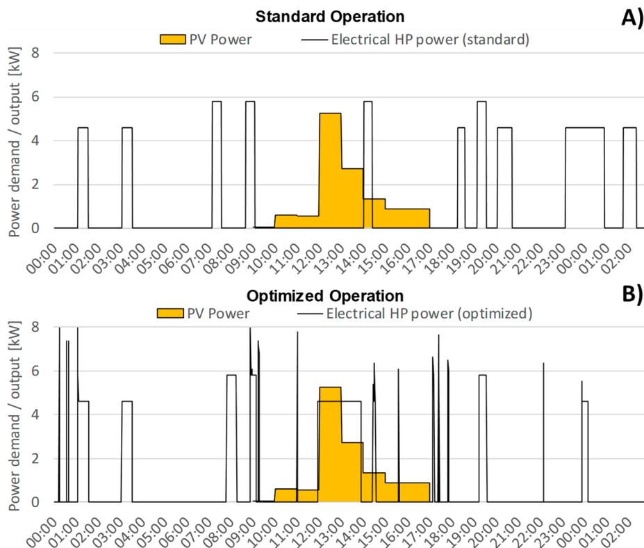
Figure 24. Standard (A) and optimized (B) heat pump operation for PV self-consumption.
