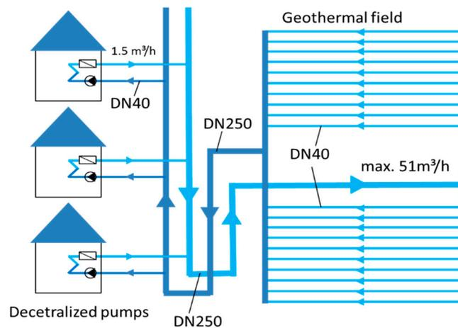
Figure 6. Hydraulic scheme of the low-temperature DHC network.
