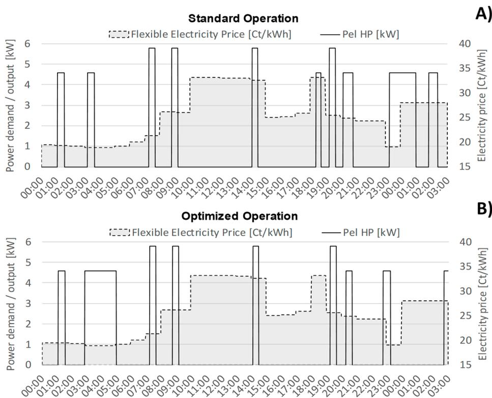
Figure 27. Standard (A) and optimized (B) heat pump operation for flexible electricity tariffs.
