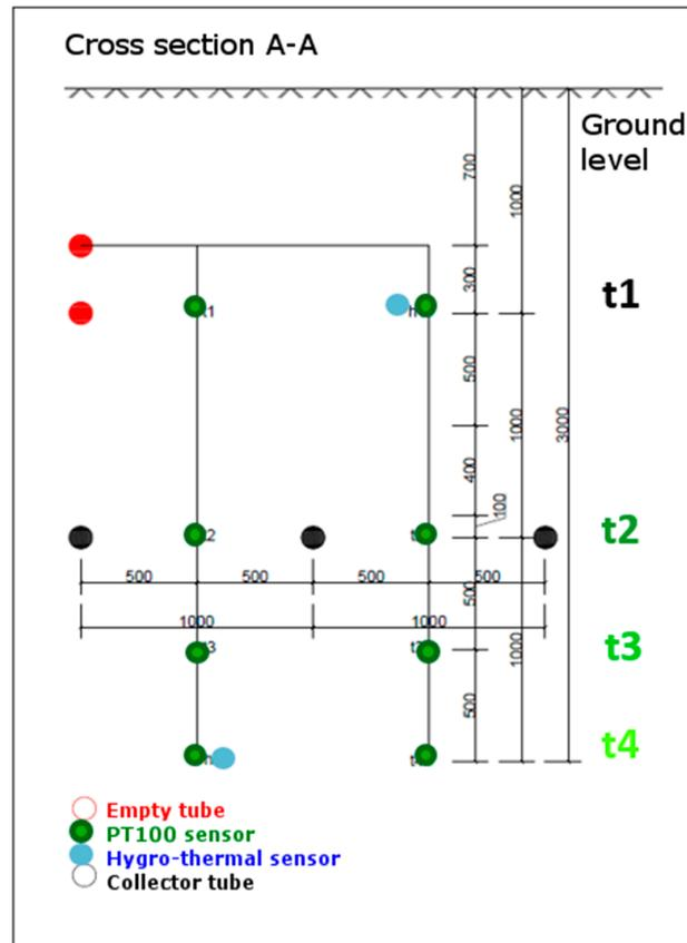
**Figure 8.** Cross-section of the measurement horizon A-A (viewing direction toward the interlocking station).
