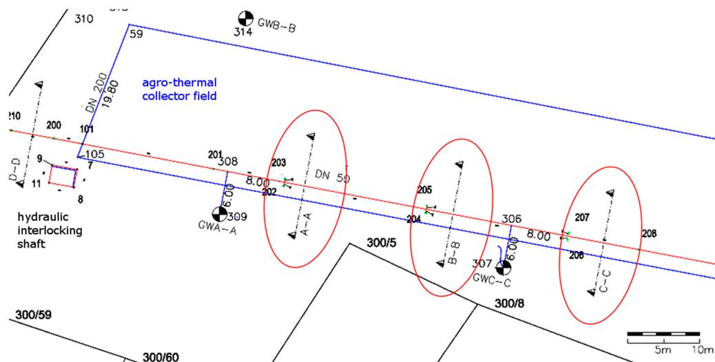
**Figure 7.** Sensor installation along one collector line.
