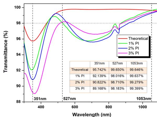
Figure 7. Transmission spectra of the dual-layer consolidated coating system with (different PI concentrations) and without PI (theoretical simulation).
