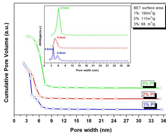
Figure 2. N<sub>2</sub> adsorption–desorption results of HRI coatings with different photoinitiator (PI) concentrations.
