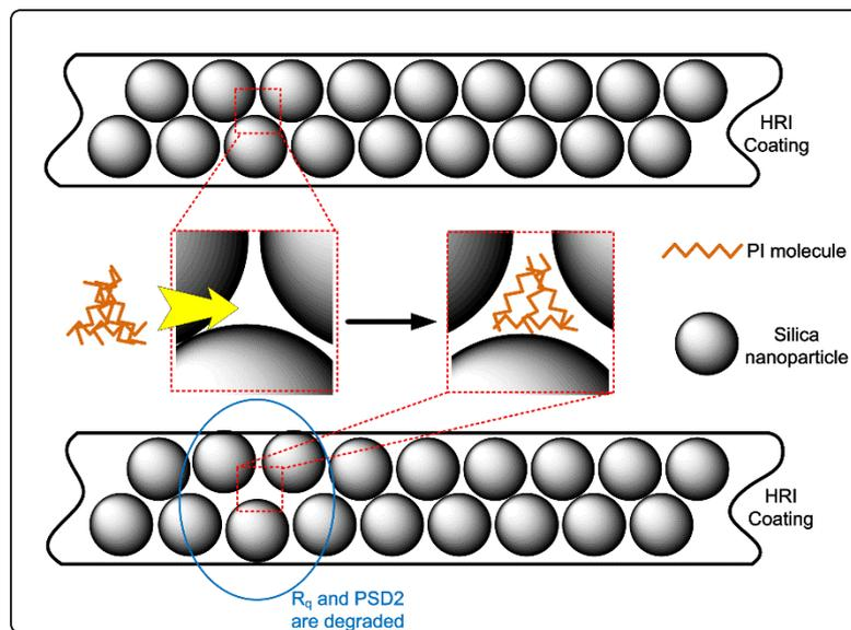
Figure 6. Schematic diagram of HRI coating deformation due to PI addition.
