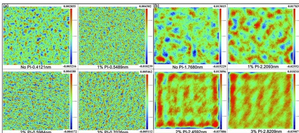
**Figure 5.** (a) Surface roughness and (b) power spectral density (PSD)<sup>2</sup> of HRI coatings with different PI concentrations.
