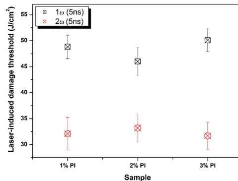
**Figure 4.** 1 $\omega$  and 2 $\omega$  laser-induced damage threshold (LIDT) of HRI coatings with different PI concentrations.
