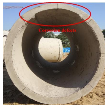
Figure 3. Simulated pipe corrosion.
