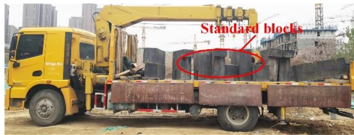
Figure 5. Full-scale traffic load.
