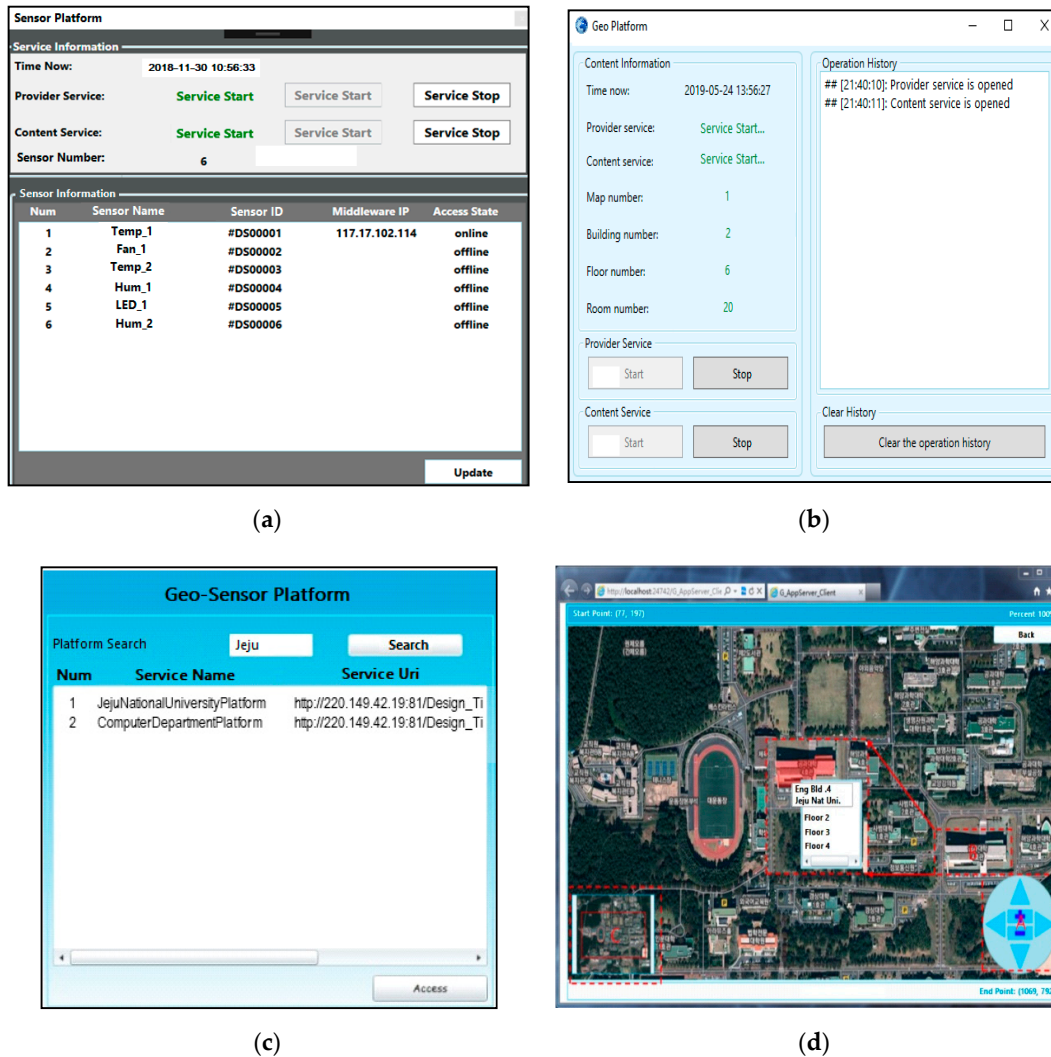
Figure 10. Geo-sensor platform service initiation deployed by the geo-sensor framework: (a) sensor platform sub-module; (b) geo platform sub-module; (c) geo-sensor platforms view; (d) selected geo-sensor platform.
