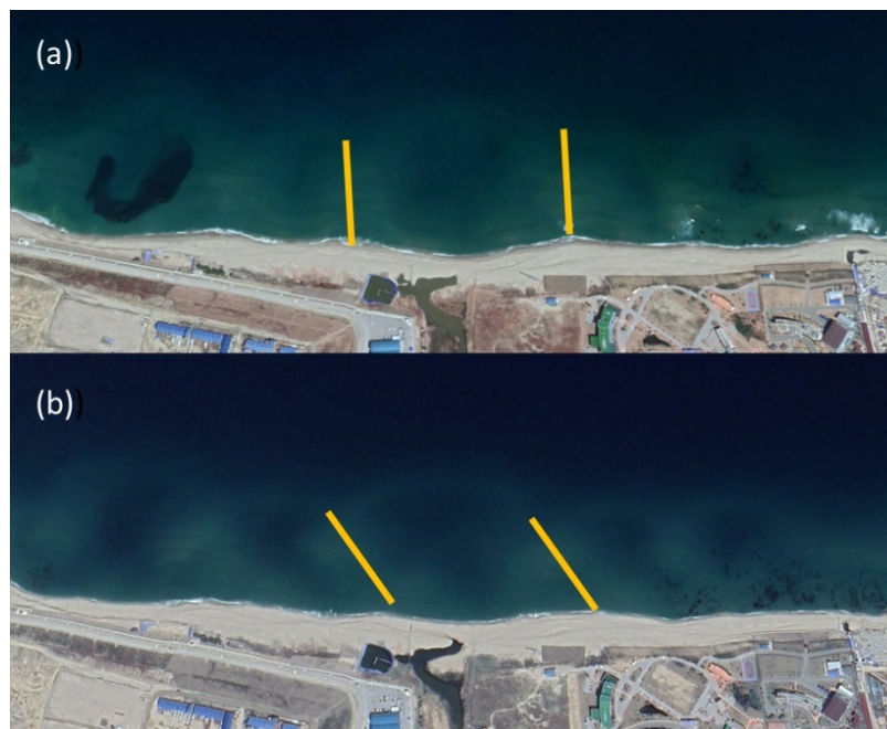
Figure 11. (a) Satellite image captured from Google Earth near L1 and L2 measured on 3 March 2018. (b) Same location but measured on 20 April 2018. The yellow lines denote the orientation of the horns of the sandbars.
