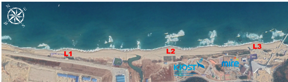
Figure 13. Satellite image captured from Google Earth near L1–L3 measured on 13 February 2019. The image shows that the waves are breaking at the locations where the sandbar horns developed, and the shoreline was advanced at the corresponding locations.
