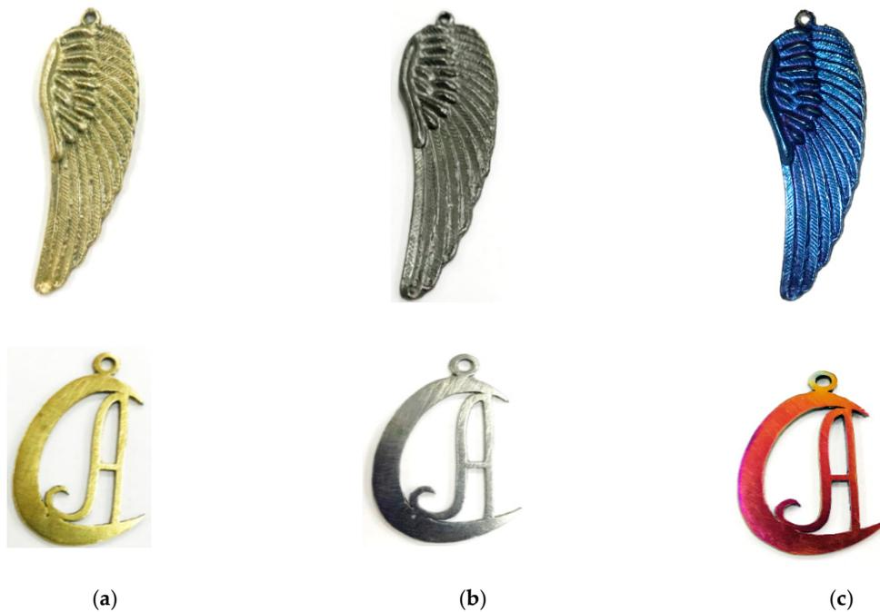
**Figure 12.** Uncoated brass pendants (a); pendants with Cr–Al–Ti–B–N coating deposited in P4 mode (b); pendants with Cr–Al–Ti–B–O–N coatings deposited in D5 and D3 modes (c).
