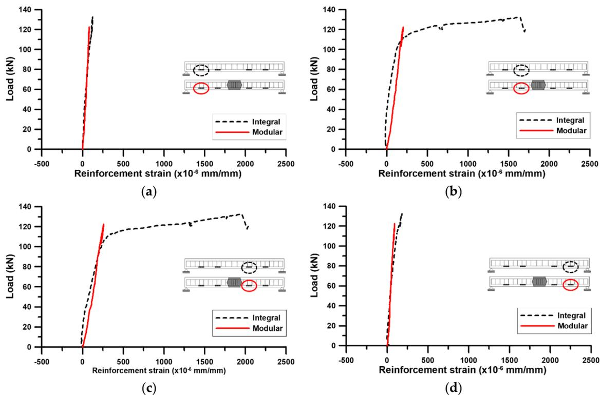
Figure 6. Reinforcement strain of the integral and modular specimens: (a) S1; (b) S2; (c) S3; (d) S4.
