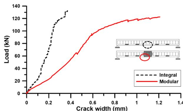
Figure 5. Crack width for the integral and modular specimens.
