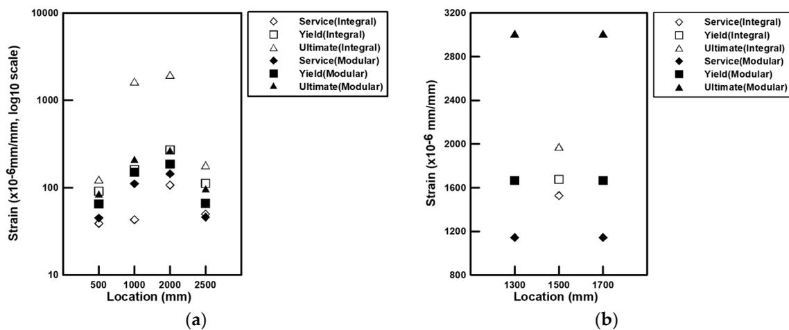
**Figure 8.** Strain change for each load stage: (a) measured strain; (b) estimated strain by EC2 Part.1-1.
