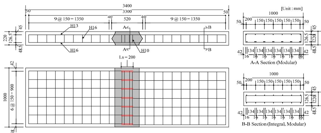
Figure 1. Specifications of the modular specimen.
