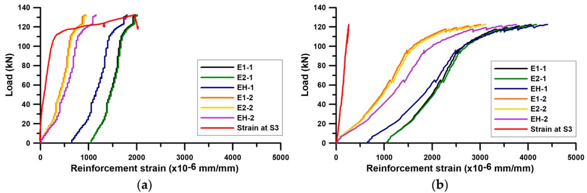
Figure 7. Estimated steel reinforcement strain: (a) integral specimen; (b) modular specimen.
