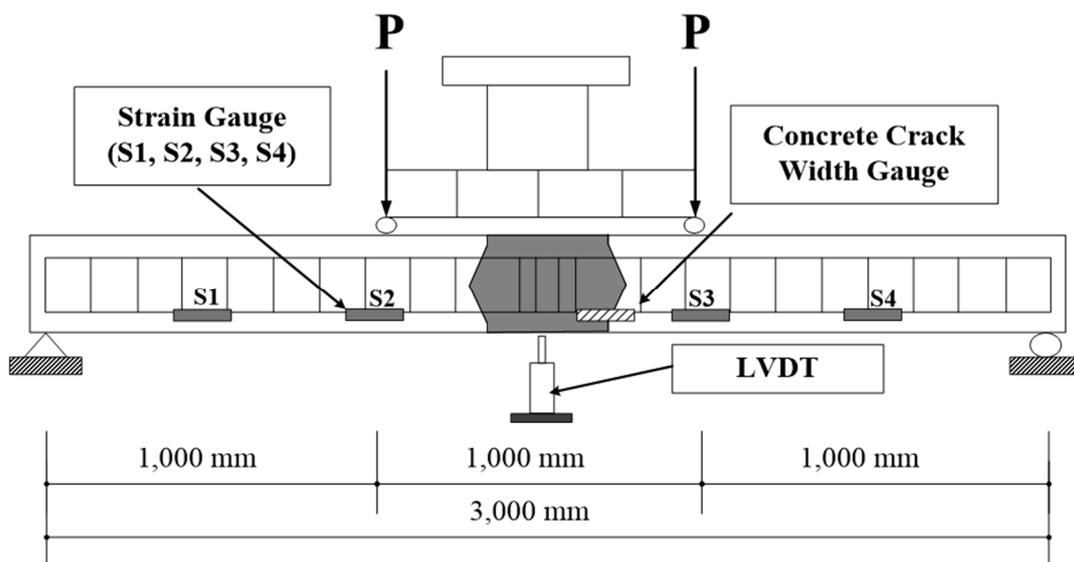
**Figure 2.** Test setup for the modular specimen.
