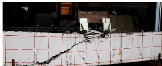
(d) Selected beam specimen subjected to two point vertical loads
