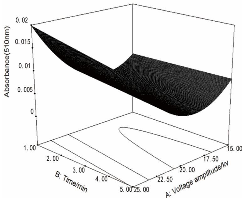
Figure 5. Response surface analysis of voltage amplitude and processing time.
