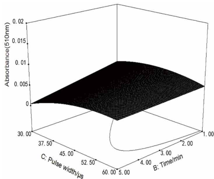
Figure 7. Response surface analysis of processing time and pulse duration.
