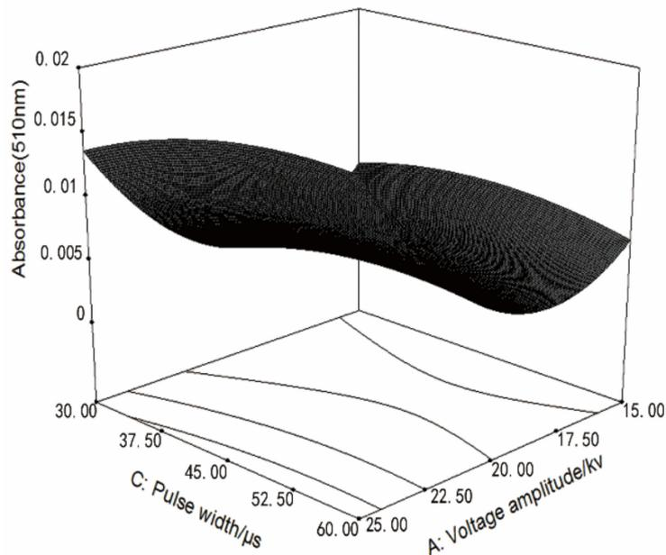
Figure 6. Response surface analysis of voltage amplitude and pulse duration.
