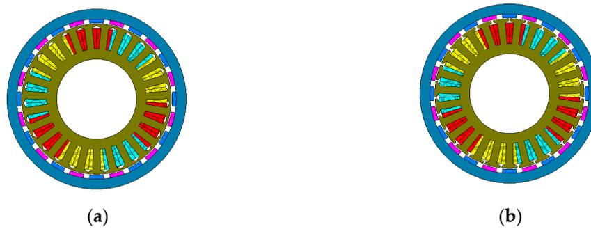
Figure 3. Finite element models of DDPMM: (a) DDPMM with open slots; (b) DDPMM with closed slots.
