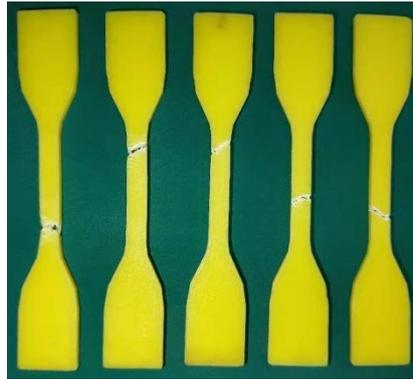
**Figure 8.** Samples after tensile testing.
