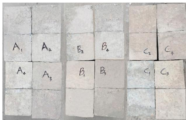
**Figure 2.** Specimens with initial crack.
