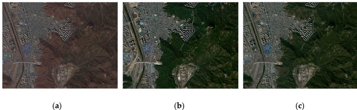
Figure 12. The experimental images for the additional dataset: (a) subject image acquired on 23 February 2017, (b) reference image acquired on 09 October 2015, and (c) normalization result of the proposed method.
