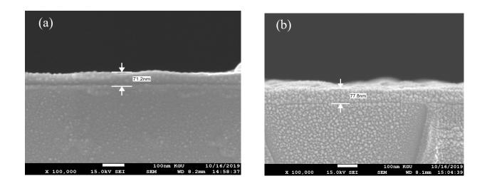
Figure S2. Cross-sectional SEM images of ZnO layer on patterned ITO glass with (a) 1SC and (b) 2SC.
