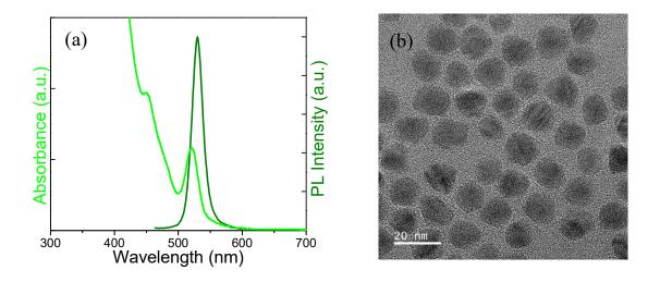
Figure S1. (a) PL and absorption spectra and (b) TEM image of CdZnSeS/Z
