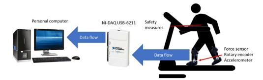
Figure 3. Experimental setup.
