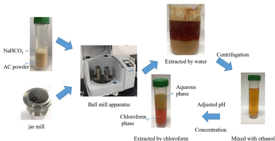
**Figure 1.** Scheme of ball mill assisted triterpenoids from the *Antrodia Camphorata* extraction method.
