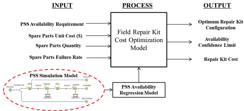
Figure 3. IPO diagram of the field repair kit cost optimization model.
