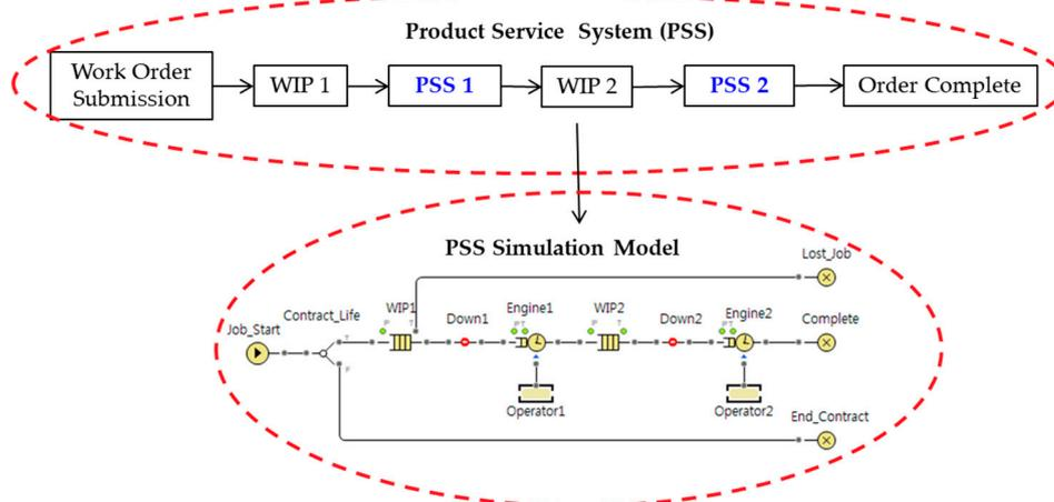
Figure 1. Simulation model flow chart for industrial printing product service system.
