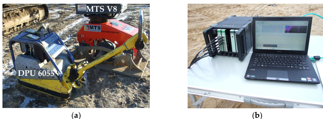
Figure 3. A view of equipment used in the research: (a) Reversible plate compactor type DPU 6055 from Wacker Neuson and hydraulic compactor type V8 from MTS; (b) Test stand.
