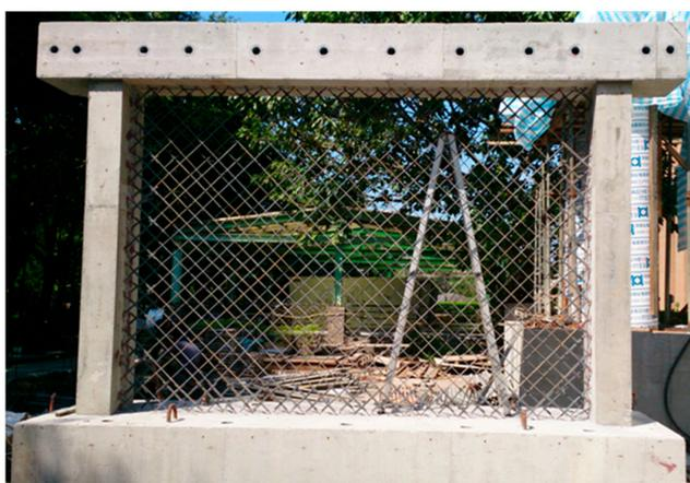
**Figure 1.** RC frame and the reinforcement arrangement of the post-installed wall of RCW1.
