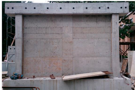
Figure 2. The front view of the specimen RCW1.
