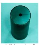
a) #1 deep and small hole standard, diameter:  $\phi$ 3 mm, depth: 80 mm
