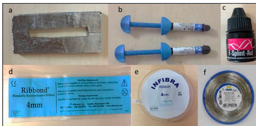
Figure 1. Experimental materials: (a) Metallic mold, (b) Flowable composite resin syringes, (c) F-splint-Aid®, (d) Ribbond®, (e) InFibra®, (f) Morelli® Ligature wire.
