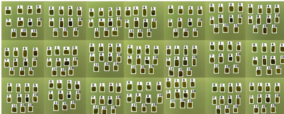
**Figure 12.** Illustration of some training data set. The white boxes in each image stands for defective beans marked by bean-picking experts.
