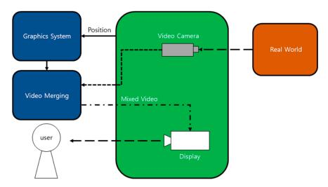
Figure 3. System Scenario of the Video See-Through Method.
