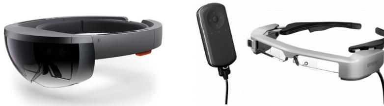
**Figure 1.** Recent Augmented Reality Devices (**Left:** Microsoft HoloLens, **Right:** Epson Moverio).
