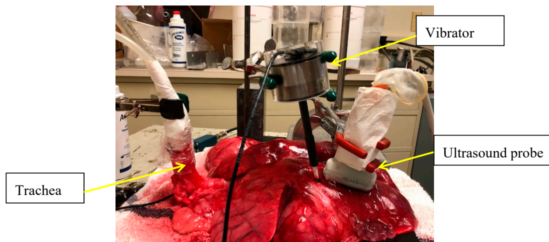
Figure 1. Experimental design for testing the surface wave speed on an ex vivo fresh swine lung. The swine lung was tested on a table. A thick rubber pad was placed between the lung and the table to reduce wave reflection. The water was injected into the lung through a plastic tube connected to the trachea of lung. In this ex vivo swine lung study, the surface wave propagation was generated using a small vibrator and measured using an ultrasound probe.
