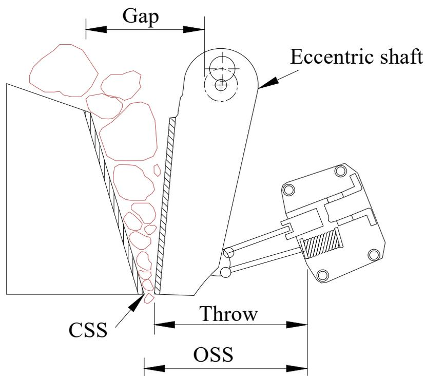
Figure 1. Kinematic of a single jaw crusher [3].
