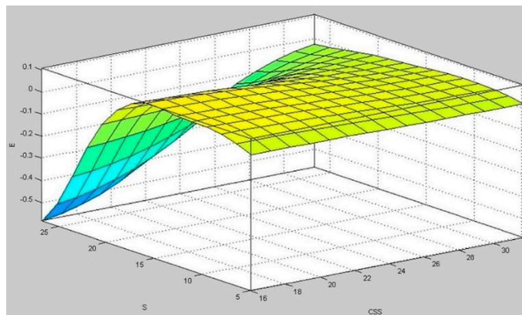
Figure 6. Energy (E) in relation to change of closed side set (CSS) and strength (S).
