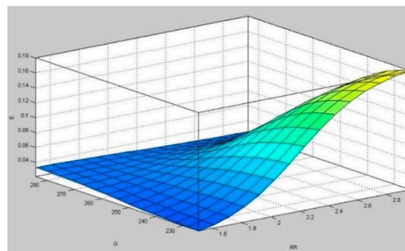
Figure 7. Energy (E) in relation to change of gape (G) and the reduction ratio (RR).
