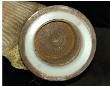
Figure 12. Bearing before the test.
