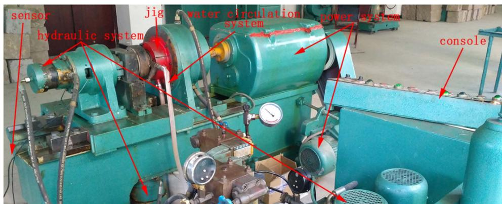
Figure 6. High-speed bearing testing machine.
