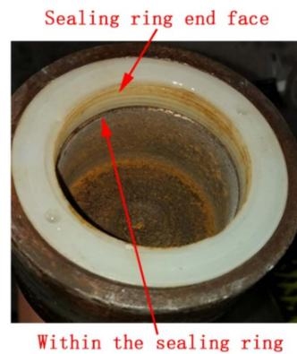
Figure 13. Bearing after the test.
