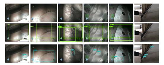
**Figure 8.** The first line is pictures of the original aircraft structures with cracks. The second line is the detection results of SSD-Mobilenet. The last line is the detection results of YOLOv3-Lite.
