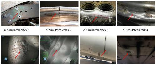
e. Aircraft structural crack 1 f. Aircraft structural crack 2 g. Aircraft structural crack 3 h. Aircraft structural crack 4
