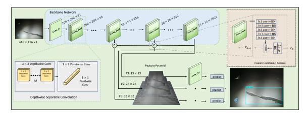
**Figure 5.** Network structure diagram of the YOLOv3-Lite model. The input is  $416 \times 416 \times 3$ . Crack featurs are extracted by the backbone network, designed using depthwise separable convolution. The feature pyramid is calculated for detecting cracks at different scales. Finally, the network outputs the detection results.
