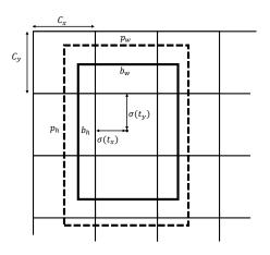
**Figure 4.** YOLOv3 predicts the width and height of the box as offsets from cluster centroids and predicts the center coordinates of the box relative to the location of filter application using a sigmoid function.
