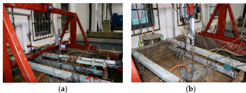
Figure 6. Bearing capacity test system of bucket foundation: (a) Horizontal loading test system; (b) Vertical loading test system.
