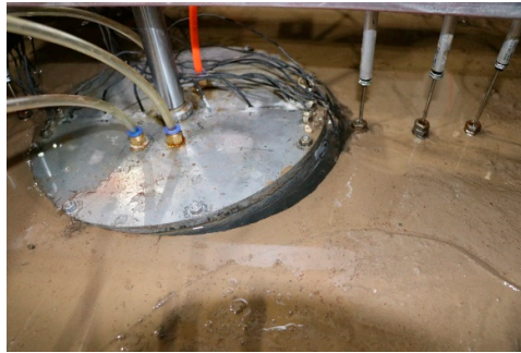
Figure 15. Failure mode of horizontal load.
