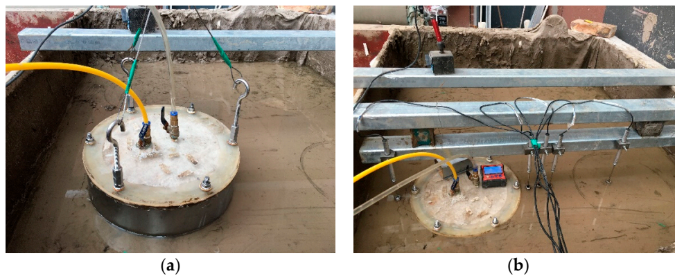
Figure 7. Installation of bucket foundation: (a) Self-weight installation; (b) Suction installation.
