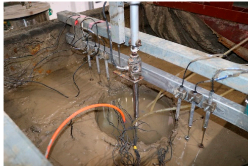
Figure 13. Failure mode of vertical load.
