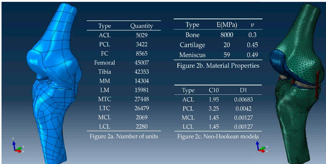
**Figure 2.** Mesh generation and material properties of knee models. The right figure represents assembled knee model. In the left figure, different colors define the different material properties. ACL: anterior cruciate ligament; PCL: posterior cruciate ligament; FC: femoral cartilage; MM: medial meniscus; LM: lateral meniscus; MTC: medial tibial cartilage; LTC: lateral tibial cartilage; MCL: medial collateral ligament; LCL: lateral collateral ligament.
