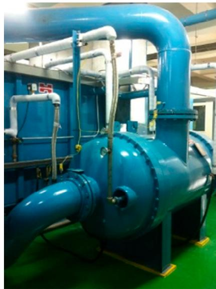
**Figure 3.** (a) Schematic drawing of closed loop nitrogen circulation; (b) photograph of the developed nitrogen cooling system.
