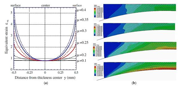
**Figure 23.** (a) equivalent strain through sheet thickness for varied friction coefficients [144], (b) the equivalent plastic strain contours obtained at 300 °C for different roller/sheet friction coefficients [147].
