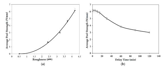
**Figure 3.** (**a**) Variation in average peel strength of Al strips vs. surface roughness [38], (**b**) variations in average peel strength vs. delay time [38].
