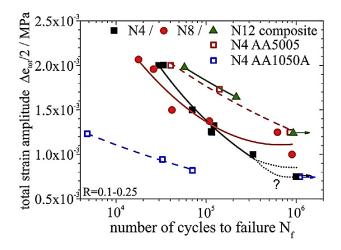
**Figure 21.** Total strain fatigue life diagram of the composites processed by different numbers of ARB cycles, ARB processed AA1050A and AA5005 mono-material sheets [137].
