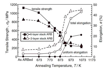
**Figure 7.** Changes in mechanical properties with annealing temperature of IF steel processed by three cycles of six-layer stack ARB compared to the results of a two-layer one [52].
