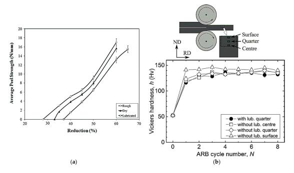
**Figure 6.** (a) Average peel strength versus the reduction in three frictional conditions, i.e., rough, dry and lubricated surface conditions [32], (b) Hardness of ARBed 4N-Cu with and without lubrication [50].
