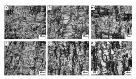
**Figure 4.** Optical microscope (OM) images of the Ti (**a**–**c**) and Cu (**d**–**f**) peeled surfaces, roll-bonded at the different thickness reductions of 44% (**a**,**d**), 56% (**b**,**e**) and 62% (**c**,**f**) [44].
