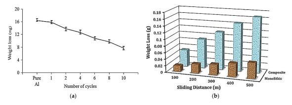
**Figure 20.** (a) Wear behavior of ARBed Al/SiC<sub>p</sub> nanocomposites processed by different rolling cycles, (b) wear behavior of monolithic material and seven-cycle ARBed Al/Al<sub>2</sub>O<sub>3</sub> composite versus sliding distance [127].
