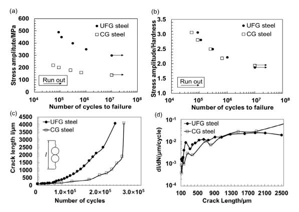
**Figure 22.** Up, (**a**) S-N curves of CG and UFG steels. (**b**) Number of cycles to failure plotted against stress amplitude normalized by hardness [138]; bottom, FCGR curves of the two steels at the same ratio between stress amplitude and hardness. (**c**) Crack length versus the number of cycles. (**d**) Crack growth rate versus crack length [138].
