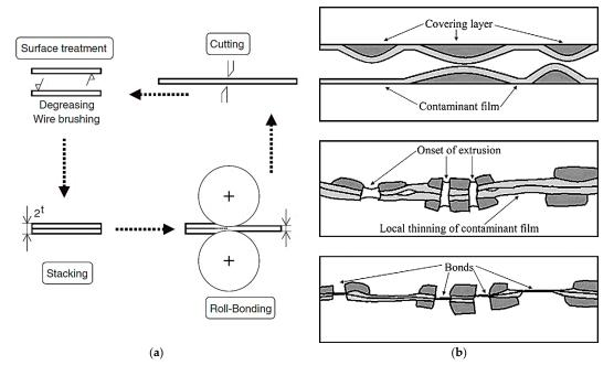
Figure 1. (a) Schematic illustration of principles of the accumulative roll bonding (ARB) process,(b) Schematic illustration of fracture and extrusion of surface layer during ARB.
