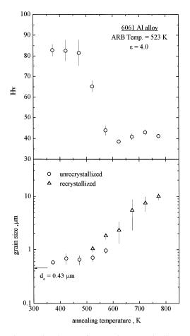
**Figure 15.** Grain size and microhardness of ARBed 6061 Al alloy under different annealing temperatures [116].
