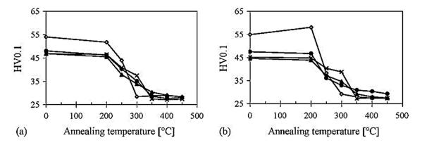
**Figure 16.** Hardness versus the annealing temperature of ARBed Al-Fe-Mn-Si sheets with (**a**) two cycles, (**b**) six cycles at 250 °C ( $\blacksquare$ ), 300 °C ( $\blacktriangle$ ) and 350 °C (×) and in cold-rolled condition ( $\diamondsuit$ ) [117].
