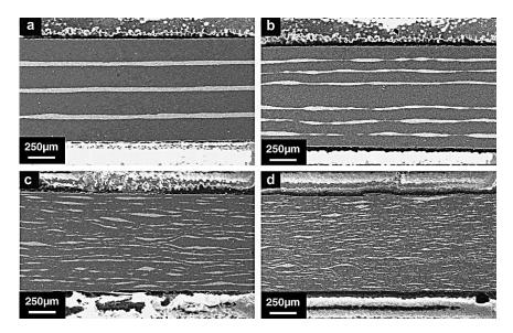
**Figure 13.** Scanning electron microscope (SEM) micrograph of ARB processed Al/Cu composite cross sections (**a**) primary sandwich, (**b**) 1st cycle, (**c**) 2nd cycle and (**d**) 5th cycle [84].
