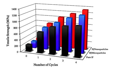
**Figure 10.** Tensile strength of ARBed pure IF steel, composite and nanocomposite versus number of cycles [60].
