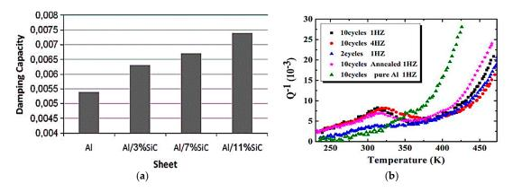
**Figure 17.** (**a**) First mode damping capacity of sheets with different percent of reinforcing agent [120]. (**b**) Damping capacity of Al/LLZNO<sub>p</sub> composites at different temperatures and ARB cycles [121].
