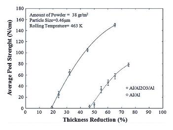
Figure 9. Average peel strength versus the thickness reduction [54].
