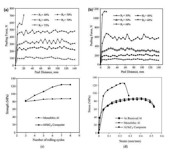
**Figure 8.** Variation of peeling force in ARBed Al-1050 strips, (**a**) in presence and (**b**) in absence of SiC particles [53], (**c**) tensile strength of composite and monolithic samples versus number cycles and (**d**) stress–strain curve of as received and ARBed samples after seven cycles [53].
