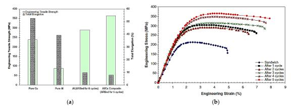
Figure 12. (a) Yield strength and total elongation of Cu, Al, ARBed Al, and ARB Al/Cu composite,(b) engineering stress–strain curves for ARBed Al/Cu composite with cycles [84].
