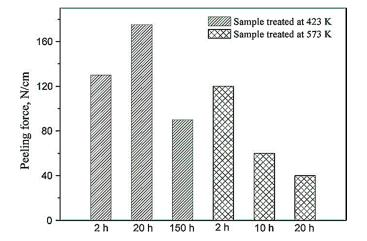
**Figure 11.** Peeling force of Cu/Al/Cu clad sheet with different heat treatment temperatures or times of heat processing [11].
