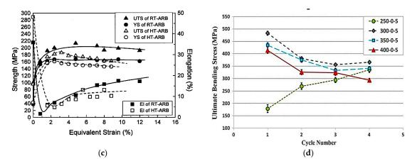
**Figure 5.** (a) Variation in diffusion layer width with rolling temperature for ARBed Al/Ti sheets [45], (b) Influence of both rolling temperature and roll speed on bond toughness of Al strips [42], (c) Variation of ambient tensile properties of 8011 alloy with increasing the equivalent strain in RT-ARB and HT-ARB samples [46], (d) Ultimate bending strength of the ARBed Al/AZ31 at different temperatures [47].
