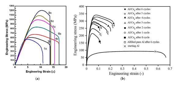
**Figure 14.** (a) Variation of stress–strain curves of the ARBed Cu/Zr materials versus ARB cycles; elongation increases up to six cycles [91], (b) engineering stress–strain curves for starting Al, ARBed pure Al after sixth cycle and Al/Cu<sub>p</sub> composite within different cycles of ARB process [97].
