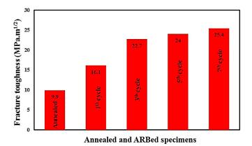
Figure 18. Plane stress fracture toughness of the ARBed Al 1050 specimens for different cycles [122].
