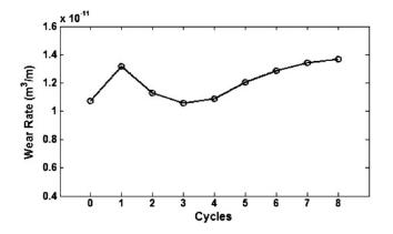
Figure 19. Variation of wear rate versus number of ARB cycles [125].
