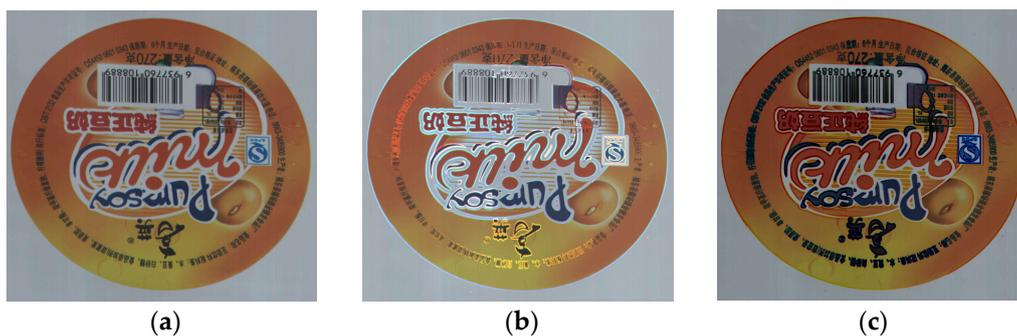
**Figure 10.** Illustration of template images. (a) reference image; (b) bright image; (c) dark image.
