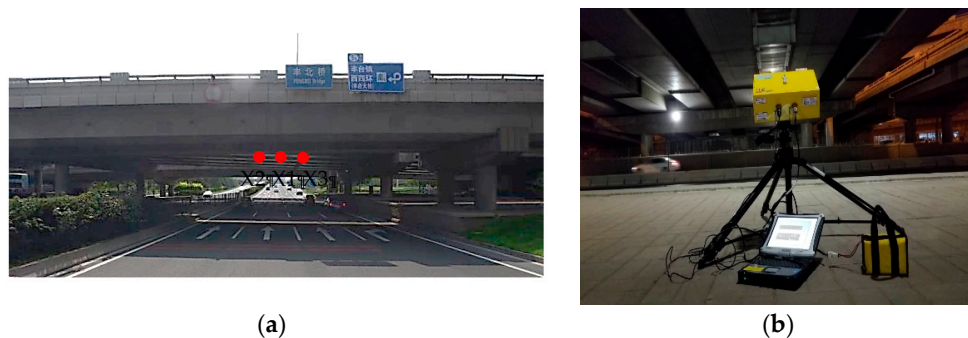
Figure 6. The Fengbei Bridge and the IBIS-S instrument layout. (a) The Fengbei Bridge and (b) the dynamic deflection measurement of the Fengbei bridge using IBIS-S.
