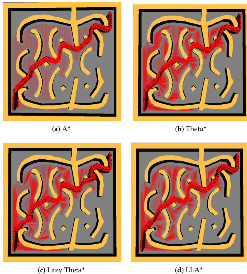
Figure 9. The planning results for an animated character using A* (a), Theta* (b), Lazy Theta* (c), and LLA* (d) on Maze #1. The extension details and final composite moving trajectories are shown in red color.
