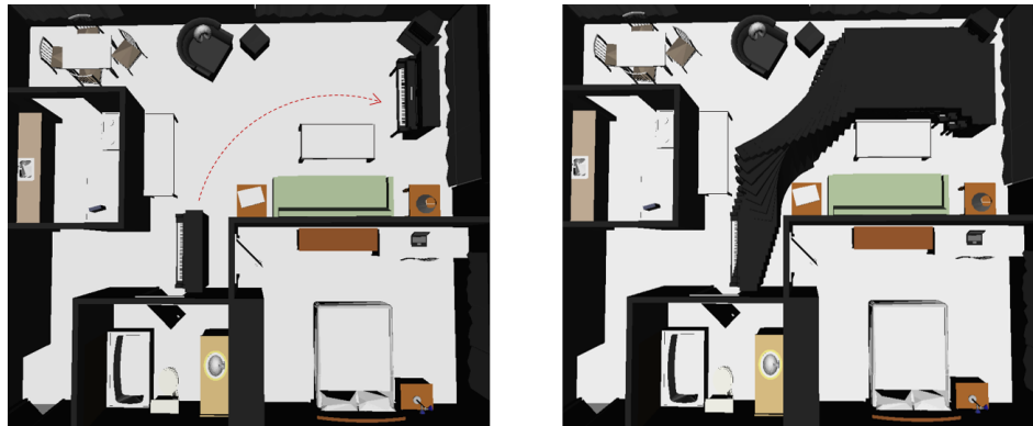
Figure 1. Moving a piano from one corner to another corner using the LLA* algorithm (top view). The left figure shows the start place and the goal place of the piano (from the left corner to the right corner). The right figure shows the composite moving trajectory of the piano without touching the tables and chairs.
