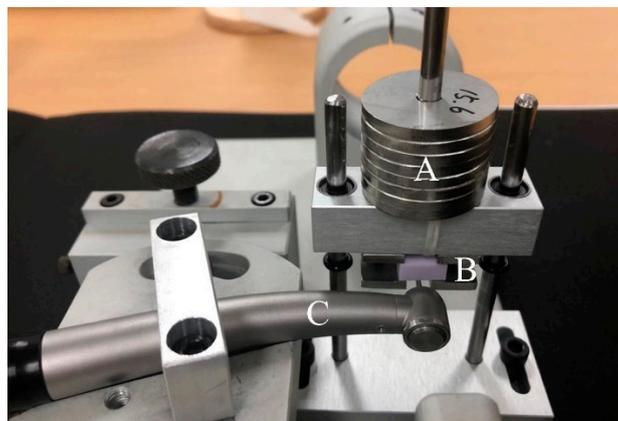
**Figure 3.** The experimental custom-made device: **A.** weight for constant load, **B.** specimen, **C.** high-speed handpiece.
