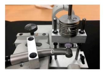
**Figure 3.** The experimental custom-made device: **A.** weight for constant load, **B.** specimen, **C.** high-speed handpiece.
