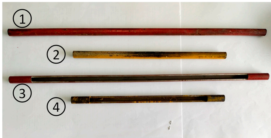
Figure 4. Intact rod (Rods 1 and 2) and damaged rod (Rods 3 and 4, with 50% cut-off of the cross section).
