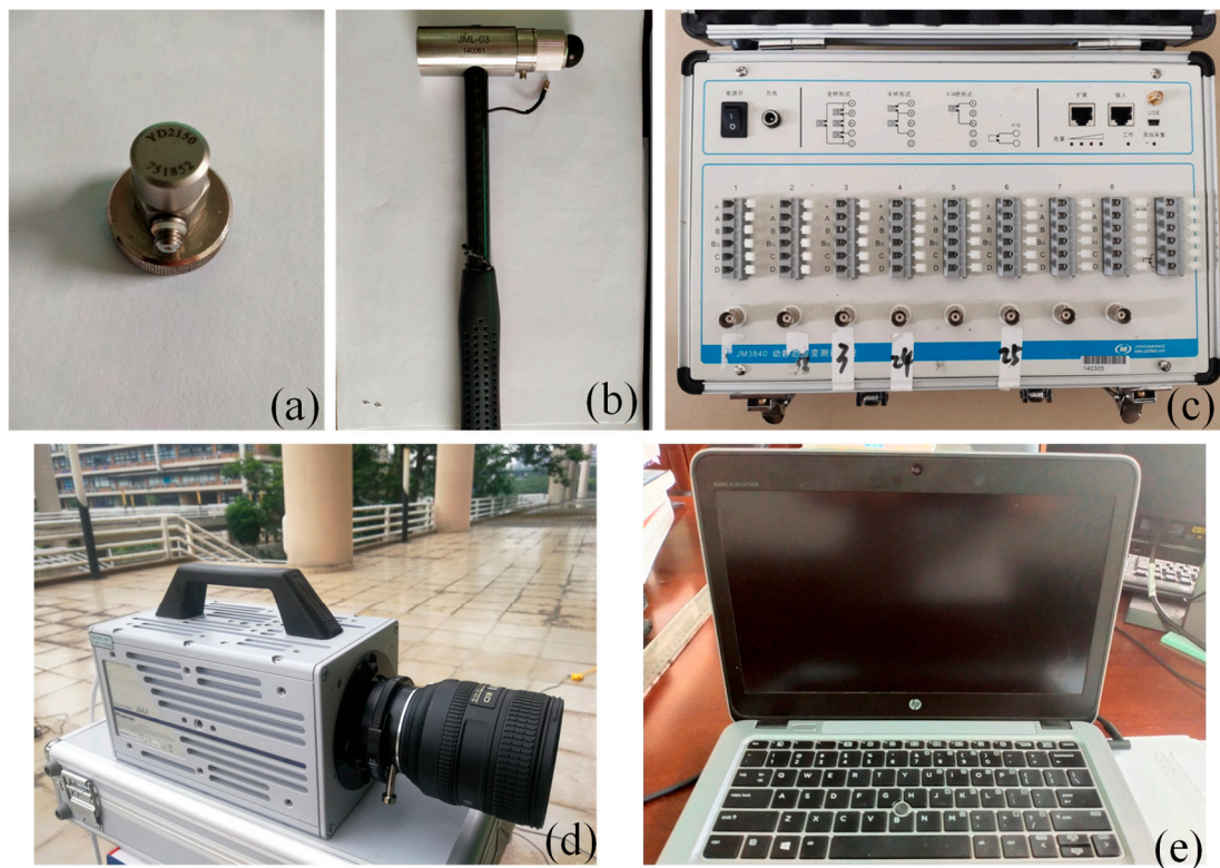
Figure 2. Experimental facilities. (a) accelerometers; (b) hammer; (c) JM3840 dynamic data acquisition instrument; (d) FASTCAM SA3 high-speed camera; (e) laptop.
